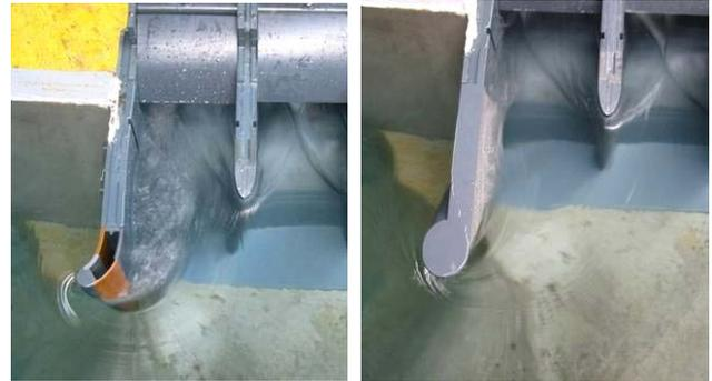
Figure 3 Flow behavior at the left bay of the gated spillway for a vertical wall (initial geometry, left) and an inclined wall (right)
