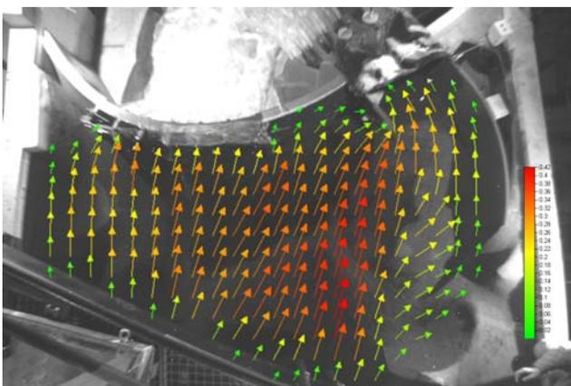
Figure 2 Velocity field in the reservoir for  $Q_{1000}$ , measured with "Particle Image Velocimetry"
