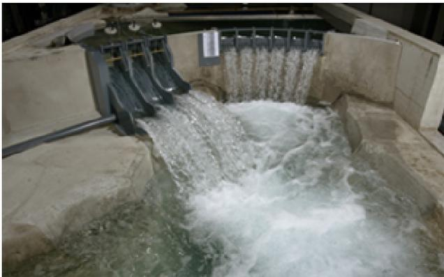
Figure 1 Physical model representing the reservoir, the dam, the spillways and the plunge pool
